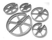
These are a single cover spacer, which can be used for both insitu' piling and diaphragm wall reinforcement. Both the light and heavy duty styles feature a central clip, which simplifies the fixing process; and allows the spacer to rotate freely around the rebar. The heavy duty spacers have a wide rim width to provide stability in poor ground.
